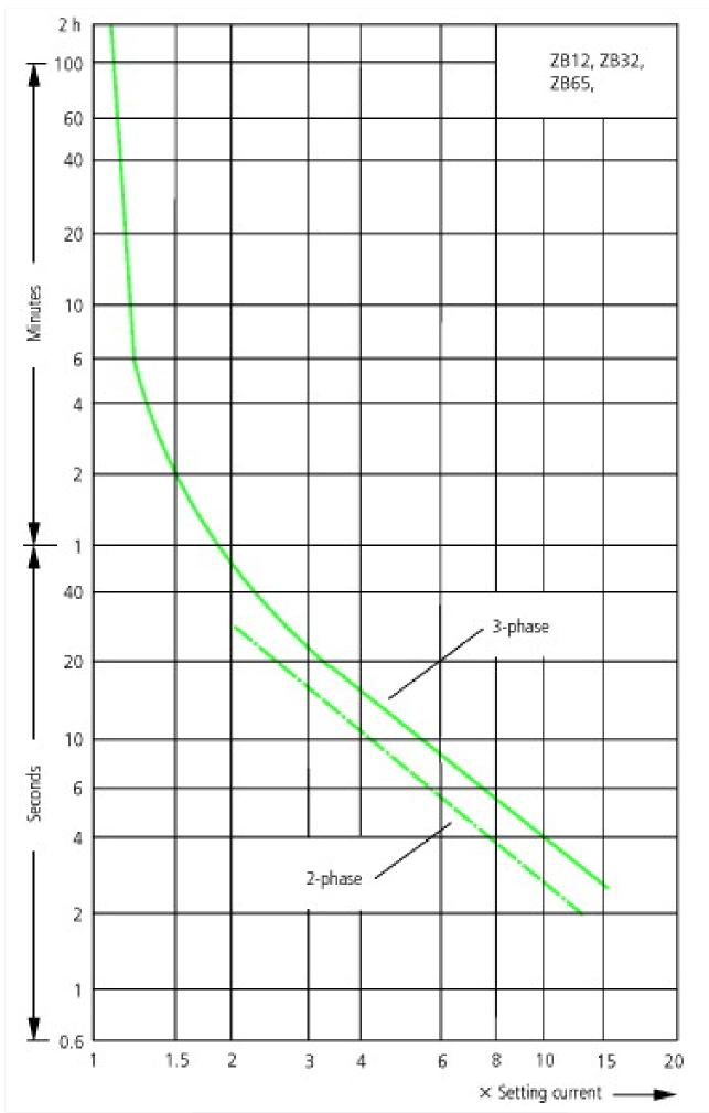
These tripping characteristics are mean values of the spread at 20 °C ambient temperature in a cold state. Tripping time depends on response current. On devices at operating temperature the tripping time of the overload relay drops to approx. 25 % of the read value. Specific characteristics for each individual setting range can be found in the manual.
