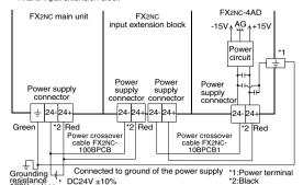
2) Connection example to the external power supply
