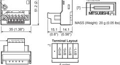
[1]Terminal block mounting screws [2]Output LED BY0 LED : The LED is lit when BY0 is on
