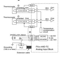
\*1: The compensating cables that can be used for connecting with the thermocouple are the following. Type K: KX-G, KX-GS, KX-H, KX-HS,WX-G,WX-H,VX-G Type J: JX-G, JX-H
